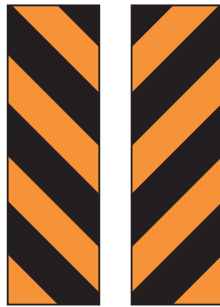
Hazard to left Hazard to right
